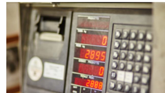
Electronic weighing of 100% of vehicles before delivery and written weight certification for end customer.
